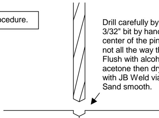
Drill carefully by twisting a 3/32" bit by hand into the center of the pinhole but not all the way through. Flush with alcohol or acetone then dry. Fill hole with JB Weld via tooth pic. Sand smooth.
