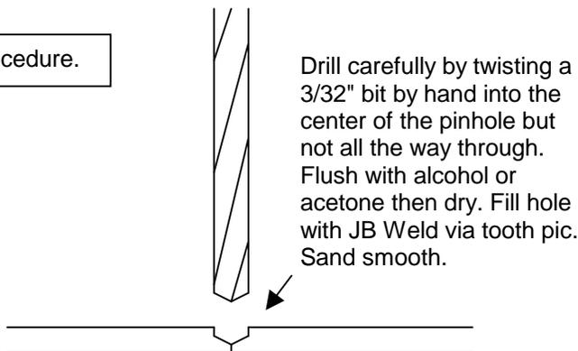
Drill carefully by twisting a 3/32" bit by hand into the center of the pinhole but not all the way through. Flush with alcohol or acetone then dry. Fill hole with JB Weld via tooth pic. Sand smooth.
